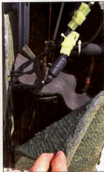
Figure 4 — With tie wraps removed, twist the wire bundles tightly and install ferrite beads. [Bob Lee, W0GXA, photo]
